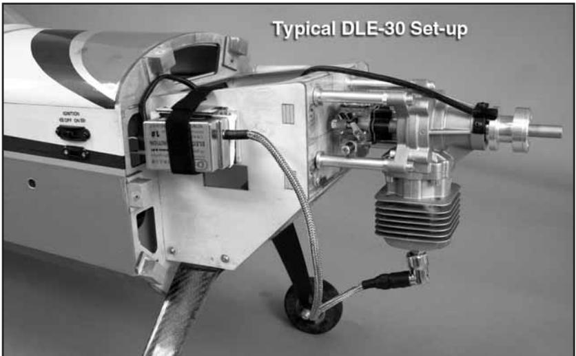
6. Connect the ignition wire from ignition module to the spark plug.
