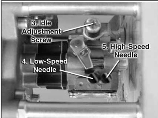
**5. (H) High-speed Needle** (adjusts the fuel/air mixture at high speeds)
