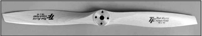
1. Remove the cowling from the aircraft. Use the included propeller washer to mark the centering hole on the propeller
