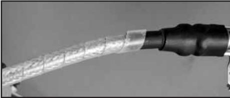
8. Install the silicone ignition wire cover over the ignition wire to the spark plug.
