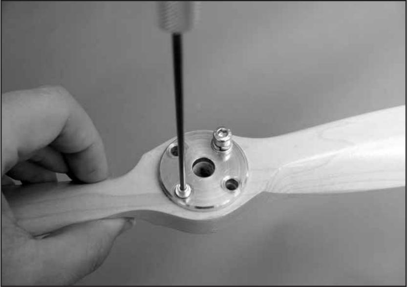
**7.** Use one of the 4x35mm SHCS with 4mm lock washers and flat washers to align the propeller washer on the propeller and use the Dead Center Hole Locator to mark the position of the remaining holes.
