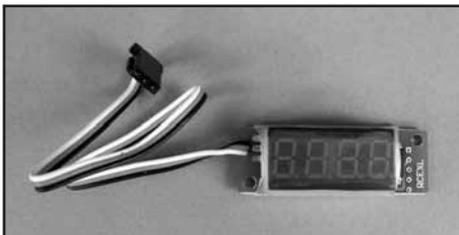
An optional Digital Tachometer is available that can be directly connected to the ignition and display the RPMs of the engine. This unit can be installed on the aircraft or used to spot check the Engine RPMs. Do not install
