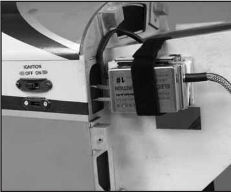
6. Install the ignition module and battery securely in the airplane forward area. It is recommended that a thin piece of foam rubber is placed between the module and the mounting surface and that Velcro® is used to hold the module in place.
