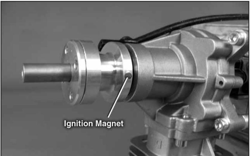
3. Next, set the engine at the top of the compression stroke. Note the position of the ignition magnet with engine inverted.
